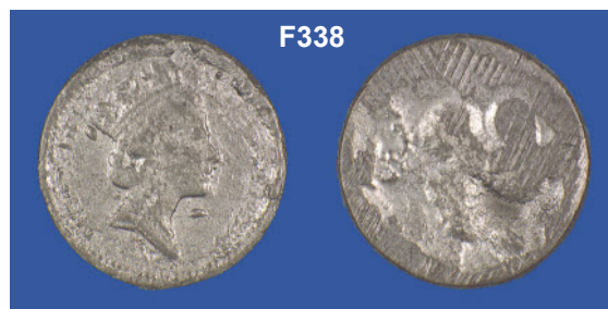
F338 - We collected this coin in 1994. Here you can see that the counterfeiter has started to imprint one side of a genuine coin into this mould. Still very poor and some filings needed to make it work in a vending machine.
