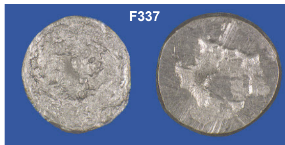
F337 - This one is made from a molten lead/tin alloy. One side has been filed so that it will fit into the entry slot of a vending machine.
