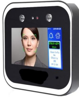
The EvolveFace 5 is an employee face recognition terminal with time and attendance that can also be used for access control to a secure area.
