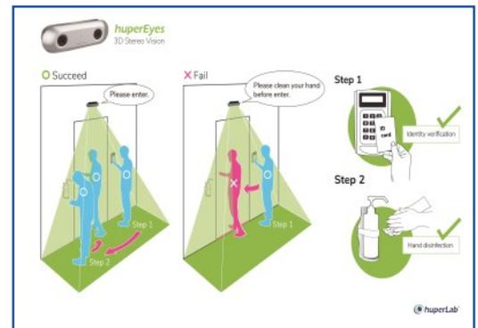
The 3D depth-sensing technology can achieve the high accuracy level to 98% with high tolerance to light and shadow changes, and the overlapping of moving objects.
