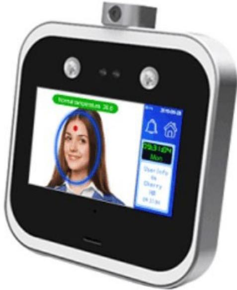
The EvolveFace 5T is a face recognition terminal with temperature detection and time and attendance function.
