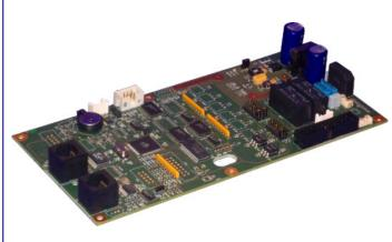
Our Coin Payment Solution control board V2, has been design to connect all the components needed to make a fixed free payment systems for pedestrian turnstiles and gates.
